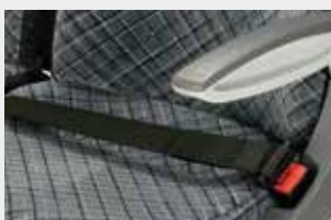
Ceinture 2 points enroulable / Retractable 2pt safety belt
