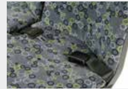
2-Punkt-Sicherheitsgurt / Retractable 2pt safety belt
