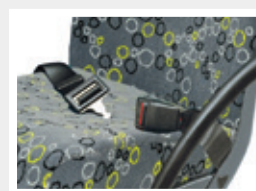
Cinturón 2pt ventral / Inertia safety belt
