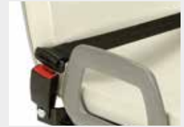
Cinturón 2pt enrollable / Retractable 2pt safety belt
