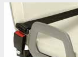
Cinto 2 pontos enrolável / Retractable 2pt safety belt
