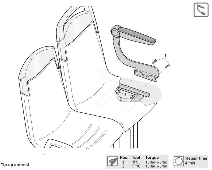
Loosen two screws (1), two nuts (2) and two washers (3) and take off armrest.
